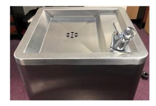
Step 4: Fit the bottle filling tap (part 6) to the 22mm hole in the rear of the bottle filling recess with the washer and brass backnut included. Fit the blue indeces to the tap button.
